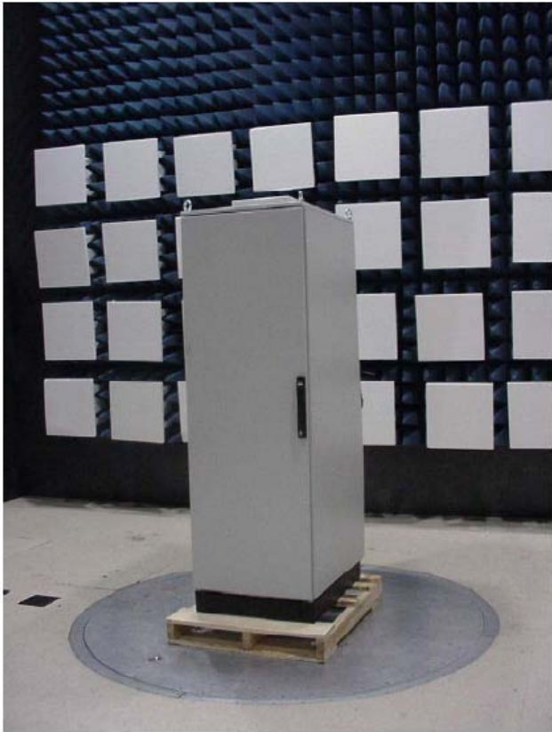
Figure 5 - Radiated Emissions Test Setup (Chamber - Front)
